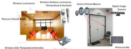
Fig. 4. IoT monitoring sensors deployed at CERTH building.
