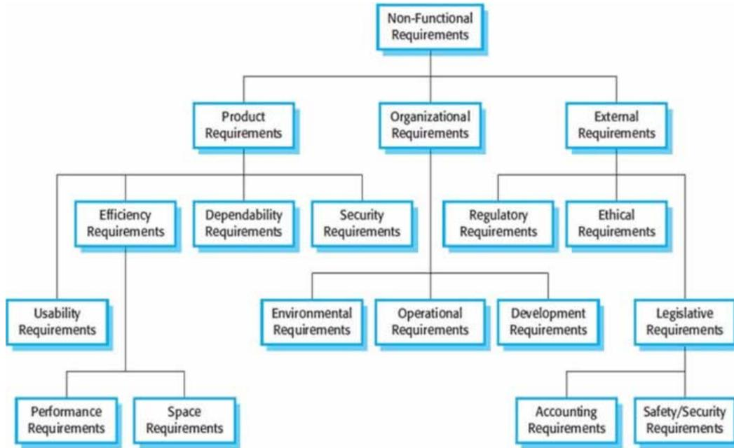
Figure 9 – Diagrammatic representation of relations between non-functional requirements (Source: Robinsce [7])
